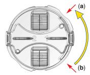
The Key is used to turn the Reading disc counter - clockwise (about 90°) until the Reading disc does not move from (b) to (a).
