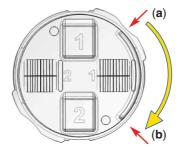
Holding the Base, turn the Reading disc clockwise until the knob of the Reading disc stops further movement from (a) to (b).
