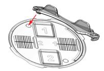
Place the Key on the assembly so that the two knobs on the underside of the Key fit into the two holes on the Reading disc.
