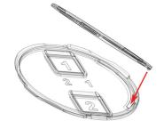
Place the lower side of the Reading disc onto the upper side of the Base, so that the small knob of the Reading disc enters the base slot.
